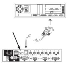
6. Power the switch back on by plugging in one of the KVM cables. The switch's front panel LEDs flash to indicate that it is in Firmware Upgrade Mode.
